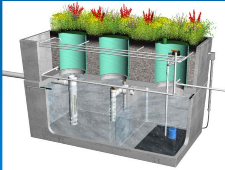
Recirculating VF wetland schematic courtesy Reactor Dynamics Inc.
