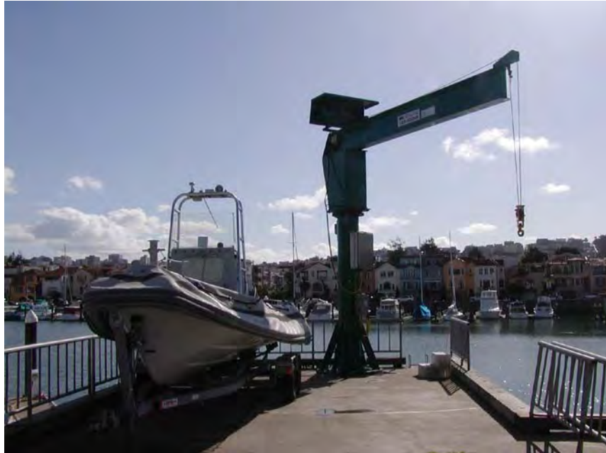
Figure 8-2, Small Craft Crane Access (Jib-boom)
