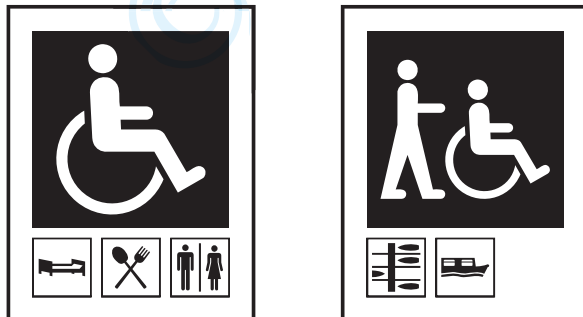
Fig. 9: Example of Two Separate Signs With Sub-Signs. Hotel, restaurant, and toilets are accessible. Assistance needed for access to piers and hire-boats.
