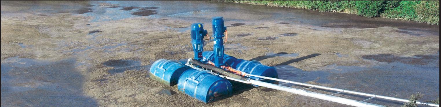
The boom attachment has a swing-around bracket system for easy servicing e.g. greasing of pump. The booms come in options of 3 to 10 metre lengths. It is of a ladder type construction which has a large 76mm O.D. effluent pipe and a 35mm O.D. service pipe for electrics.
