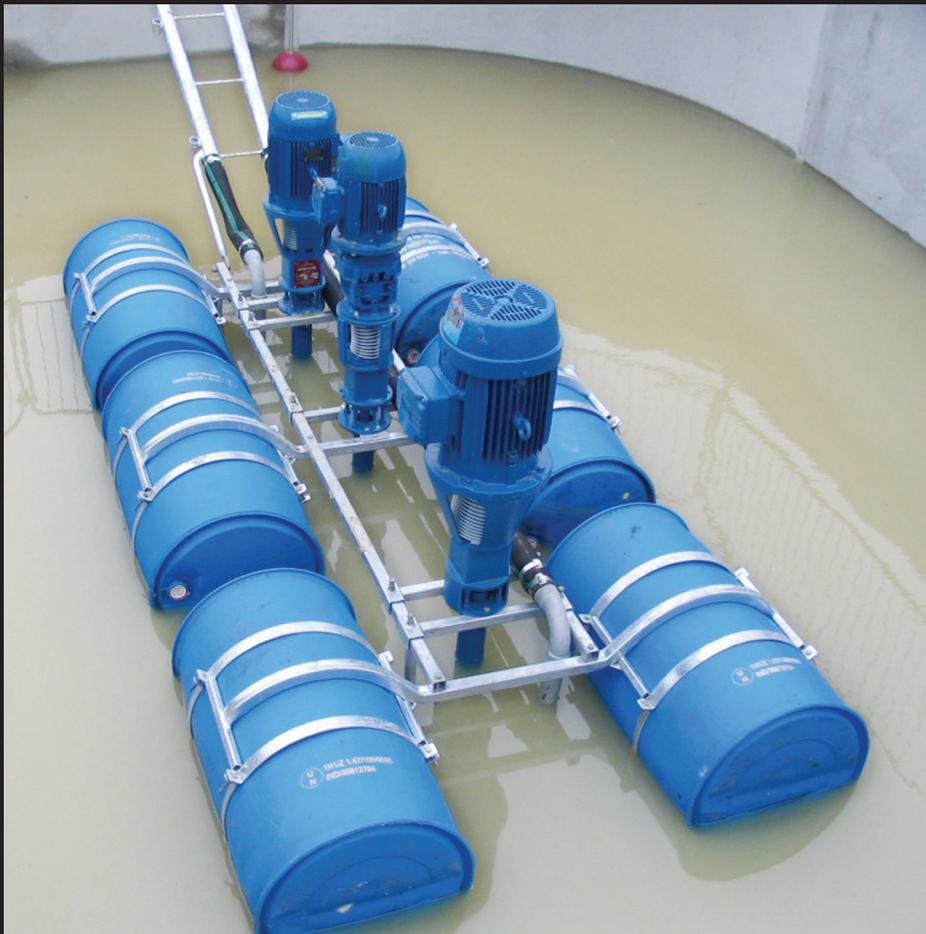
The **Williams Pump Pontoon** is a multi-drum float which allows the positioning of effluent pumps and stirrers on effluent ponds and concrete tanks.
