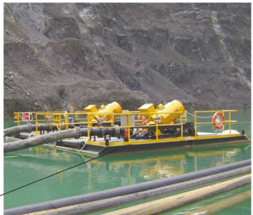
Wide pontoon with low centre of gravity
