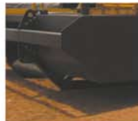
Above: View of skid runners, lifting and towing points fitted to the ME pontoon pump unit.
