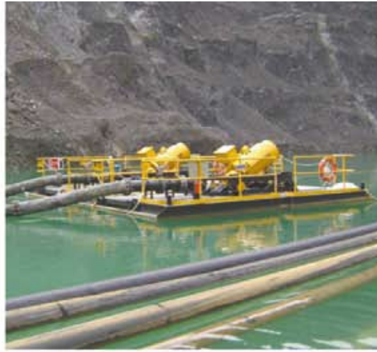
Right: A pontoon in operation at a mine in Indonesia fitted with two directly driven pumpsets.
