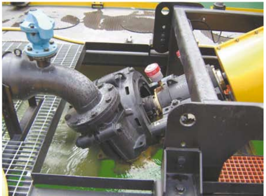
Right: Directly driven pumpset showing positioning of angled pump relative to the waterline.
