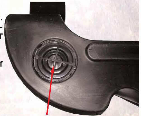
Polyfused caps to fill the foam.
